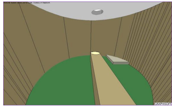
Figure 8: The circle of light cast by the roof aperture for the northern circular room at noon on the summer solstice. The view is from north looking towards the south.
