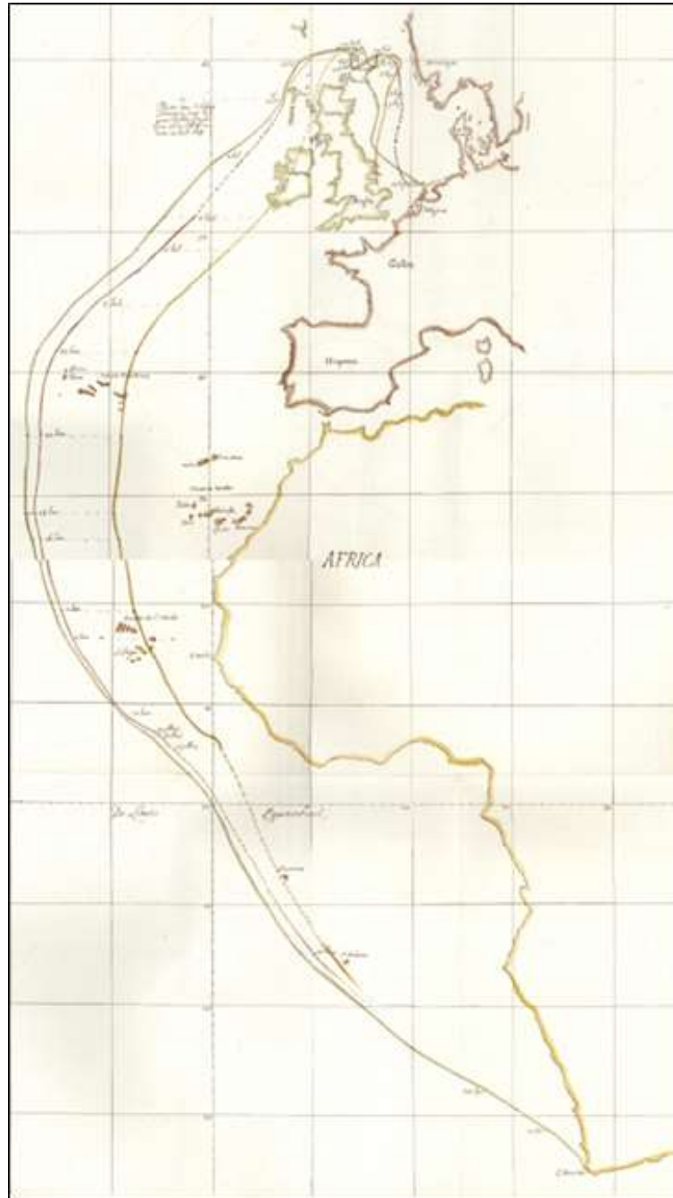
Figure 14: The route determined by the Alcmaer's navigators is indicated by the westernmost curve (green); that based on raw timing measurements is represented by the easternmost curve (yellow). Upon correction for the effects of the Earth's rotation, Huygens arrived at the curve closest to but slightly to the east of the westernmost route (red). (after Oeuvres Complètes de Christiaan Huygens , IX, 273; not in copyright).
