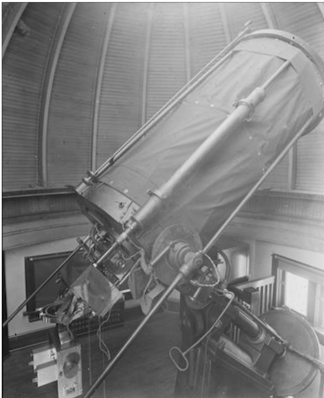
Figure 5: The rebuilt 30-inch telescope with dual channel photoelectric photometer attached. Circa 1928 (courtesy: University of Illinois Department of Astronomy).
