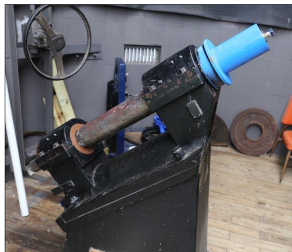
Figure 9: The Brashear equatorial head and polar axis in November 2017 as it undergoes modification for a 16-inch telescope (photograph used with the permission of David Leake).
