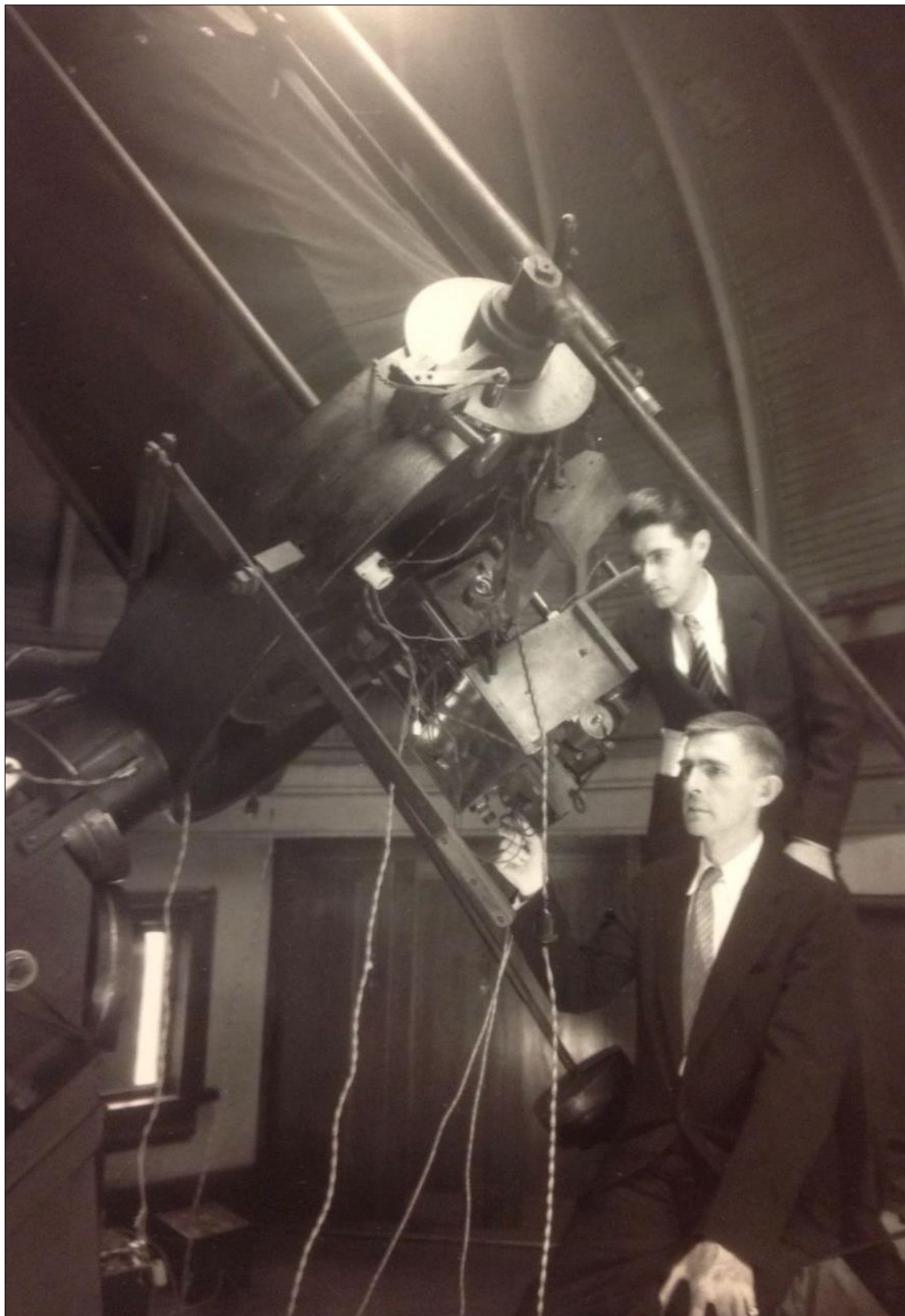
Figure 6: University publicity photograph of Robert Baker and student Harry Crull recreating the opening of the Chicago Worlds Fair on 27 May 1933. Note that the photoelectric photometer has been rebuilt into a single channel instrument using a Lindemann electrometer (courtesy: University of Illinois Department of Astronomy).
