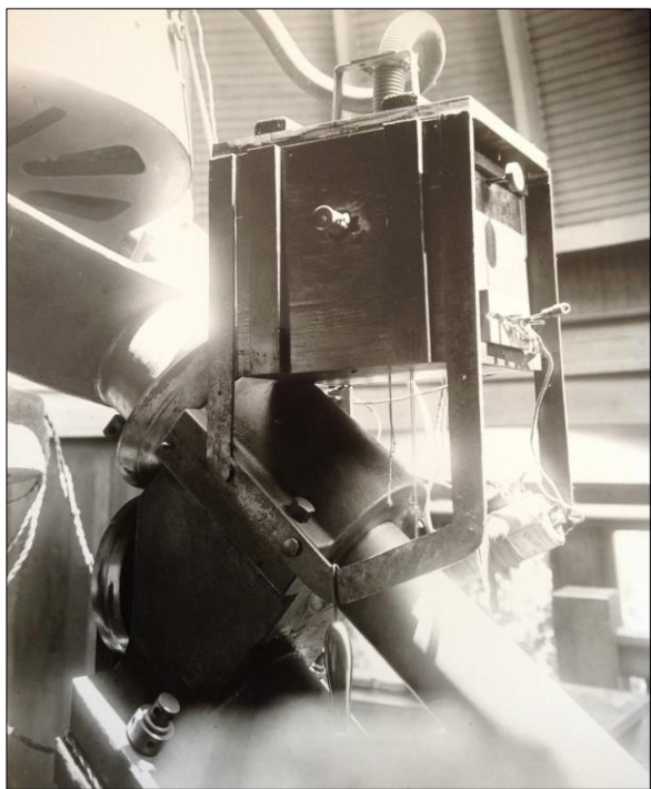
Figure 4: Electrical test equipment mounted on the right ascension axis and connected to a detector at the primary focus. Dates to circa 1917 (courtesy: University of Illinois Department of Astronomy).
