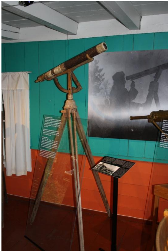
Figure 2: The homemade 7-cm refractor (photograph by the author).
